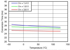
Figure 3. CONVERSION TIME vs TEMPERATURE
