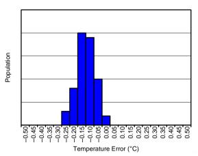
Figure 6. TEMPERATURE ERROR AT +25°C
