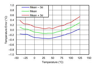
Figure 5. TEMPERATURE ERROR vs TEMPERATURE
