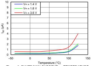
Figure 2. SHUTDOWN CURRENT vs TEMPERATURE
