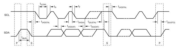
Figure 12. Two-Wire Timing Diagram
